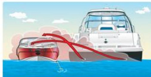
Boat exhaust can also flow back into the rear of the boat. The amount of carbon monoxide can reach life-threatening concentrations on and near swim decks.
